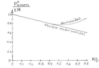
Fig. 16. The pressure at the bottom of the crest of the solitary wave according to eq. 95 of this chapter compared to the shallow water expression of chapter VIII.
