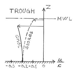
Fig. 7. Comparison of the horisontal velocity below the middle of the trough according to the Stokes' second order theory and according to the cnoidal theory of this chapter. The wave considered can be : T = 10.1 seconds, D = 8.0 metres, H = 5.4 metres. Metres. The 'trough depth is rather different according to the two theories, but the velocity at the bottom is close to the same.
