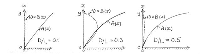
Fig. 13. In the final expression for w (eq.18) a term was neglected (eq.14). This term, B(z), is here compared numerically to the second order term, A(z), of w for three different waves. It is seen that A(z) is more than 100 times bigger than B(z) for shallow water and deep water waves, and A(z) is 10 times bigger than B(z) for transitional waves.
