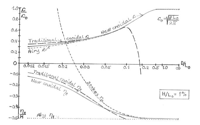
Fig. 12. Comparison of the traditional shallow water cnoidal theory, the Airy theory, and the Stokes' theory with the new cnoidal theory, with respect to the celerity and the trough depth. At the shallow water end the wave height will reach H/D = 0.8. While the traditional theories have deficiencies at one end or the other, the new cnoidal theory can be used for any D/L.
