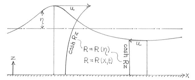
Fig. 2 In a second order wave we now want to express u as only one term with a cosh Rz distribution. This means that R must be a function of x,t instead of just a constant.
