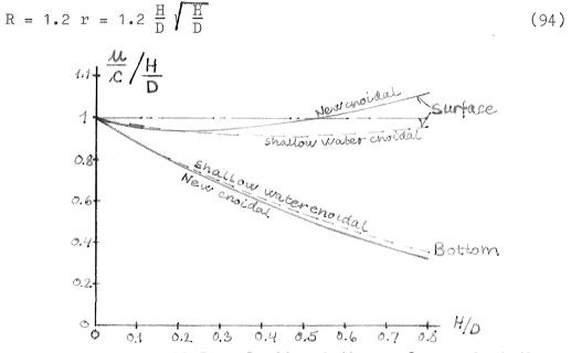
Fig. 15. The horizontal particle velocity at the surface and at the bottom of the crest of the solitary wave according to eq. 93 of this chapter compared to the shallow water expression of chapter VIII.
