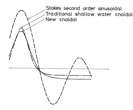
Fig.17. Using the equations tabulated in chapter X we find the shallow water limit of the new cnoidal wave slightly different from the traditional cnoidal wave, but in this appendix it is shown how to express the new wave so it will coincide with the traditional wave.
