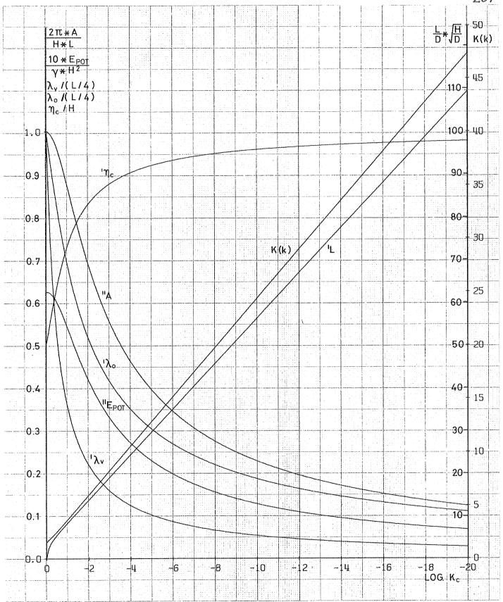
GRAPH 4. Choidal wave. As functions of log  $k_c$ : wave-length, potential energy, crest-height, crest-volume, distance from the crest to the point of inflection and to the point on mean water level, and K(k).
