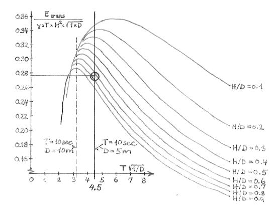
Fig. A2. Determination of the wave height. Part of graph 6.
