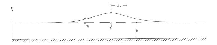
Fig.2. Definition sketch. Solitary wave. Undistorted. H/D = 0.6
