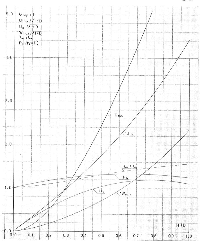
GRAPH 8. Solitary wave. As functions of the wave-height and mean water depth: particle velocities and acceleration, pressure, and the distance from the crest to the point of maximum vertical velocity.
