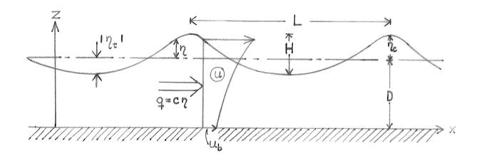
Fig. 1. In the shallow water limit the sinusoidal theory will give a parabolic velocity distribution. This can be used in second order terms to find the choidal theory.
