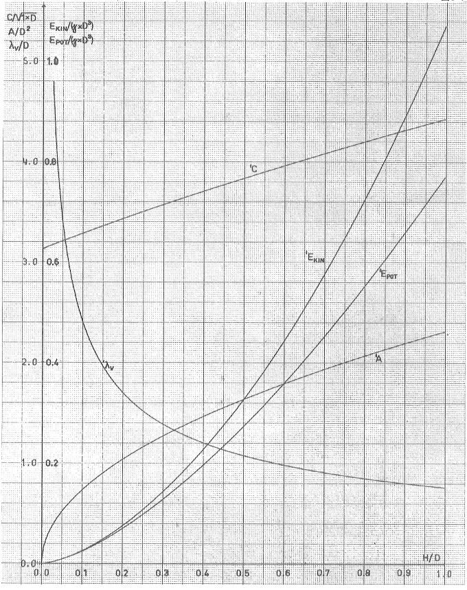
GRAPH 7. Solitary wave. As functions of the wave-height and mean water depth: celerity, kinetic and potential energy, wave volume, and distance from the crest to the point of inflection.
