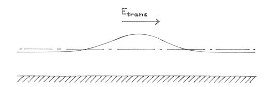
Fig. A1. The transported energy for a shallow water cnoidal wave is not just twice the potential energy.
