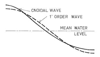
Fig. 2. Cnoidal deep water wave compared to the first order wave for H/L=10%. The second order waves in eqs. 16 and 17 will give the same profile. The perturbation solution from eq. 15 will be only slightly different.
