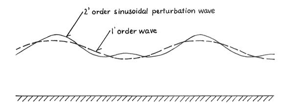
Fig. 15. The first order wave and the second order sinusoidal perturbation wave. (For deep water waves the second order wave will though never get the shown 'crest in the trough'.) The second order wave shows qualitatively how the first order profile should be changed, but a more reasonable solution than the perturbation solution should be tried.
