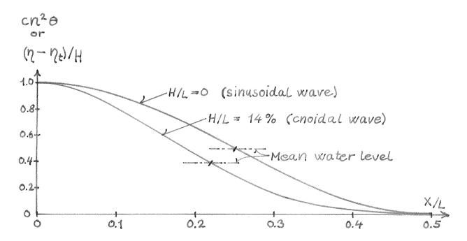
Fig. 21. The wave profile for the progressive cnoidal deep water wave of maximum practical steepness, i.e. H/L=14%, and the profile of the sinusoidal wave. For all other steepnesses the wave profile will be in between.
