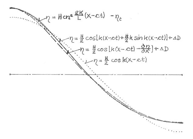
Fig.13. Comparison of different second order waves for the deep water wave with the steepness H/L = 10%. For infinite deep water the difference is not big. There is though a small difference between the two sinusoidal waves, and this is due to the influence of the third and higher order terms not considered in a second order theory. The second order wave above that is closest to the choidal wave is (incidentally) also a third order wave.
