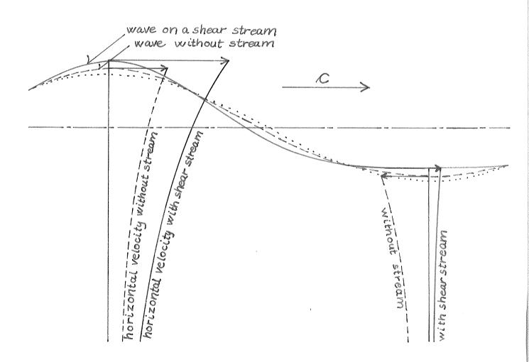
Fig. 5. Second order deep water wave propagating on a shear stream.
