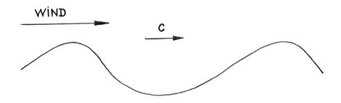
Fig. 6. During the generation of waves by the wind the pressure on the surface will not be p=o. The result will be the asymmetrical wave.
