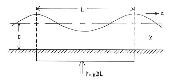
Fig. 7. At the bottom there is a dynamic boundary condition, which is as simple as shown above for the progressive wave. For progressive deep water waves it is special simple.
