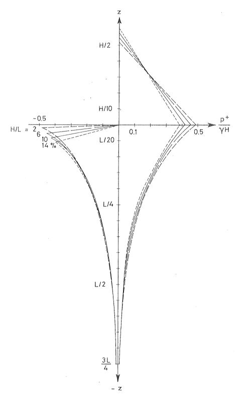
Fig. 9. Maximum positive and maximum negative wave pressure below the progressive choidal wave for different steepnesses: H/L=2%, 6%, 10% and 14%. Note that the unit is different below and above the mean water level, z=0.
