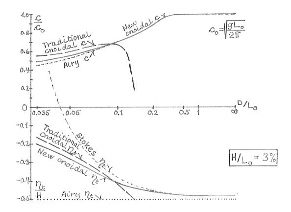
Fig.1. The celerity and the trough depth. The traditional wave theories can only be used in specified regions, as shown, while the new cnoidal theory of chapter IX can be used on any water depth.
